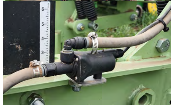
Row Control valve adjusts the flow to each individual row.
