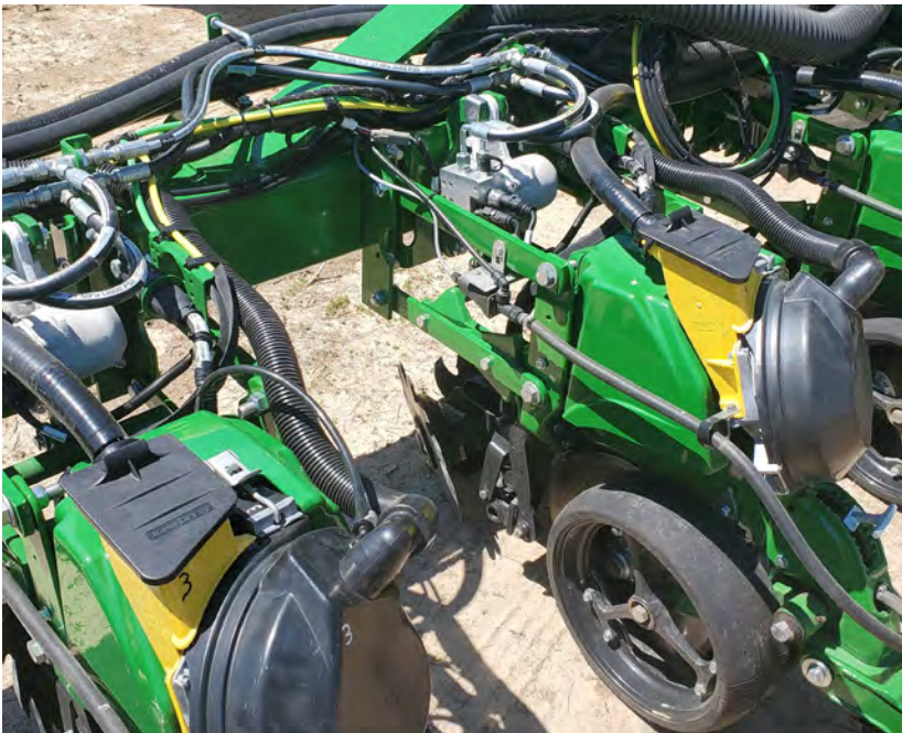
Row Control valve adjusts the flow to each individual row.
